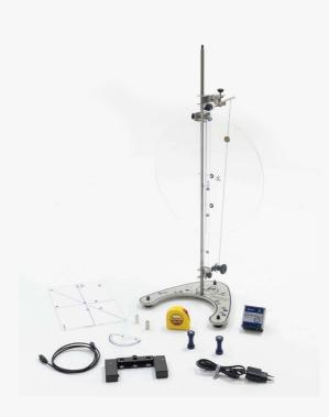
Set of simple pendulum and physical pendulums, bearing pivot, with multichronometer (Bluetooth)
