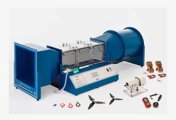
Wind tunnel with wind turbine, renewable energy, sensors and multimeters
